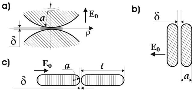
Fig. 1. Narrow gaps between (a) two metallic grains, (b) two parallel elongated grains, (c) two coaxial elongated grains.
